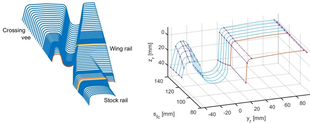
Figure 2: Successive profile slices defining the geometry for a crossing, with geometrical features connected into ‘interpolation paths’.
